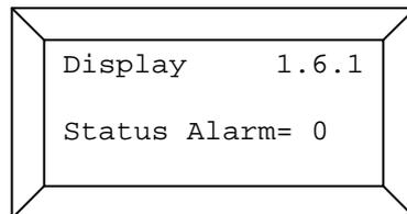
when the shadow impact module is restarted, the alarm status will return to 0.
