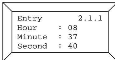
that the time you enter must be the wintertime! After you have confirmed your entry by pressing the *Enter* key, the processor clock adopts the new time data. Please double-check that the new date and time have been entered correctly.
