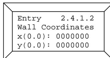
In the 3<sup>rd</sup> line enter the x coordinate (easting); in the 4<sup>th</sup> line enter the y coordinate (northing). The first index of the coordinates defines the wall number (0 – 4). The second index specifies the respective pair of coordinates concerned (0 or 1).
