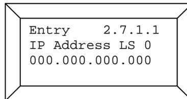
If a light sensor is removed from the wind park, the IP address should be reset to zero (default) to ensure that the shadow impact module no longer retrieves data from this light sensor.
