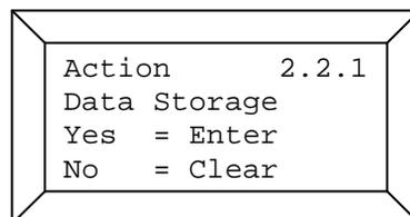
To save the data, please press the *Enter* key. To cancel the process, please press the *Clear* key. During a storage process, the shadow impact module should not be switched off.
