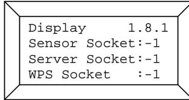
component is active. A value of > 0 means that the network connection is active.
