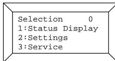
To go to the desired menu, please press the corresponding numerical key, e.g. 1 to go to the *Status Display* menu. In the second menu (2) you can configure the shadow impact module. The third menu (3) is for manufacturer setting and adjustment menus which will not be described in detail in this manual.
