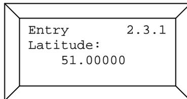
Please start by entering the degree of latitude. The degree of latitude is preset to 51.00000 degrees. Use the arrow keys to change the position of the cursor. Please confirm your entry by pressing the *Enter* key. The display will now show the entry menu for the degree of longitude.
