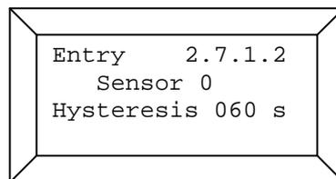
Enter the hysteresis using the numerical keys and confirm your entry by pressing the *Enter* key. Use the arrow keys to navigate through the entry positions.
