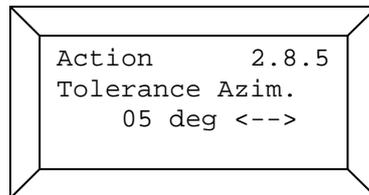
Entering the azimuth tolerance is required only if the shadow impact calculations take into account the nacelle position of the WTG. The range is 0 ° to 15 °. The azimuth tolerance reduces the calculated difference between the sun azimuth and the nacelle position measured. The higher the azimuth tolerance value set, the wider the calculated shadow impact ellipse of the rotor. Thus, the azimuth tolerance can be used to improve security regarding the shadow impact calculations.
